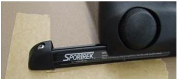
5. After all the holes are drilled, remove the roof rack from the hardtop. (**Reassemble the same as it was removed as the holes in the Side Rails may be in different locations**) Eliminate all debris and clean all of the exterior holes on the hardtop and the bottom of the Side Rails with alcohol to ensure a leak free fit. Install the (10) Foam Washers onto the Side Rails and the End Caps.
