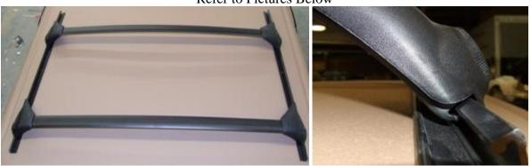
3. Measure @ 2 ½" inches from the center of the back end of the rain channel to the outer edge of the Side Rail on both sides. Then measure the rail @ 3 ½ inches from the center of the front end of the rain channel to the outer edge of the Side Rail on both sides. (**This will take several checks to assure equal alignment as movement can/will occur**) Once correct measurement is achieved, place pieces of tape on the hardtop around the Side Rails to indicate if any movement has occurred.
