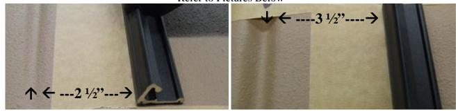
4. Give one final visual inspection before beginning to drill! Take one End Cap to use as a drill guide for the (2) front and (2) rear holes in the Side Rails. Drill a 3/16 hole. When finished drilling all holes install the End Caps temporally by sliding a #10-24x1.25 into the holes, this will secure it enough to drill the rest of the Side Rail holes (6).
