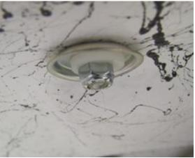
10. Install the Snap-On Covers (10) to all of the Retainer Washers. Install Stanchions and Crossbars to desired positions. (Caution be sure to tighten the Adjustment Knobs before traveling)
