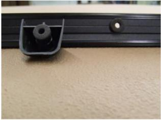
6. Place the Side Rails back on the hardtop and install the Tie Down Loops (4) on each end of the Side Rails.
