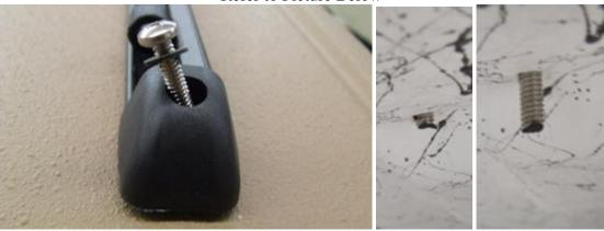
8. Install the Retainer Washer, Nylon Washer and the Nylok Nut to the bottom of the screws. Tighten using a 3/8" nut driver or socket and a drill or screw driver. Be careful not to over tighten. Refer to Pictures Below
